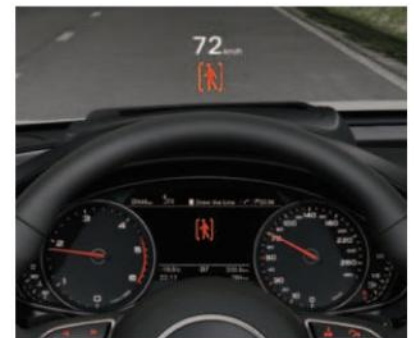
▲ The driver assistance system in the Audi Q7 has a night vision feature to help prevent hitting pedestrians.
